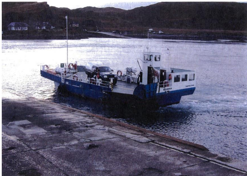
Figure 2: MV Belnahua showing the quarter loading arrangement.
