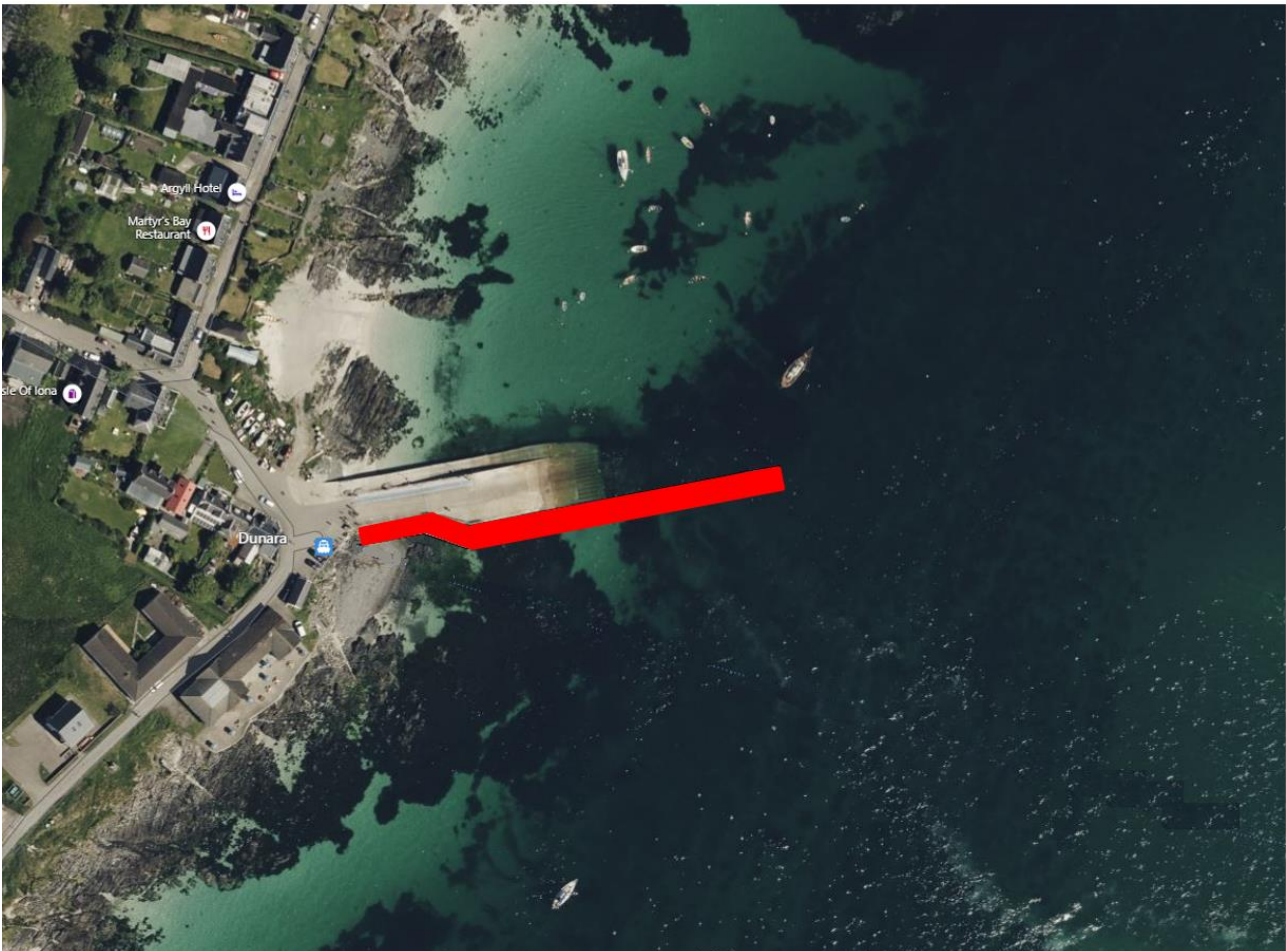
Figure 4-1 Indicative layout of pier at slipway
