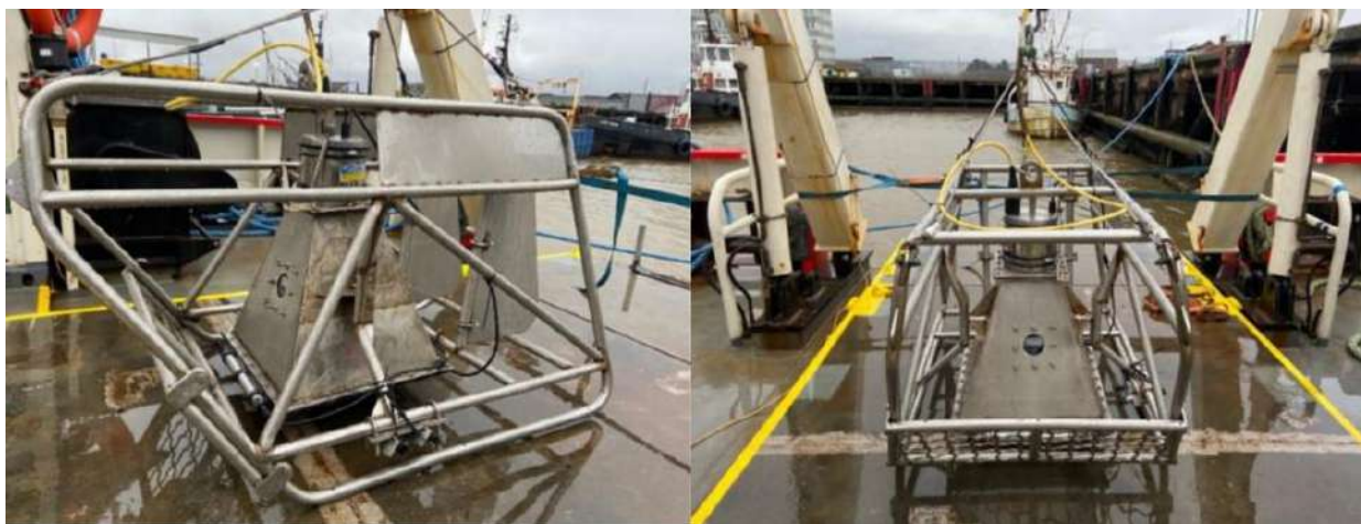
Plate 2 OEL's drop-down camera and deployment frame.
