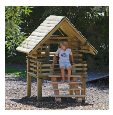
Climbing structure constructed from ø 15-21cm splinter free and sanded timber posts with angle cut to top end grain face. Attached climbing rope net and rope obstacle constructed from six strand steel-core rope in a natural colour, with aluminium swages and stainless steel ø 8mm S-clamps.
