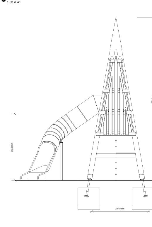
Pyramid tower constructed from ø 22-30cm de-barked posts and 3-5cm thick timber cladding, de-barked by hand. Three internal platforms constructed from 40mm tongue and groove boarding.
