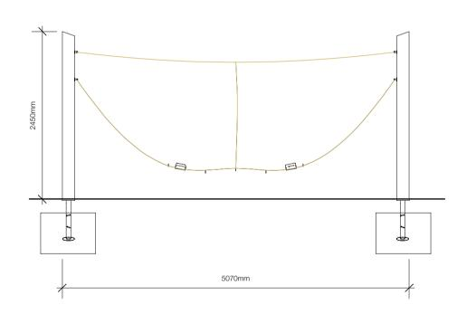
Double Hammock swing seat constructed from ø 18-21cm de-barked posts of spruce/fir, boiler pressure
