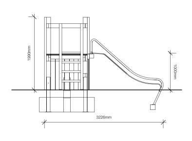
Square play hut on stilts with ladder, wide stainless steel slide and table with two integrated benches at the lower level. Constructed from sawn timbers of not impregnated mountain larch. Platform at 1m contructed from 40mm tonge and groove timber boarding Timber ladder with ø 42mm milled and mortised hardwood climbing rungs. Stainless steel slide with glass-bead blasted walls and ø 42mm handrail tube.
