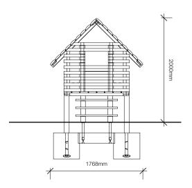
Play house on stilts with roof, steps, balcony, window cavity and internal integrated table and two benches. Constructed from sawn timbers, with externally clad roof constructed from 3-5cm timber de-barked by hand. Floor of 25mm tongue and groove boards and steps of 32mm hardwood.
