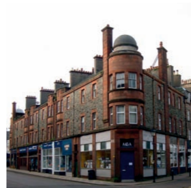
[8] Longrow South 1909 T L Watson Fine 3 storey tenement with bull faced stone work and red sandstone dressings. Circular and octagonal domed corner towers. Crenellated parapets and shallow bay windows. Keystone feature and flanking circlets in doorway lintels. Longrow South was created to sweep away the unsanitary conditions of the Wide Close which fronted Main Street.
