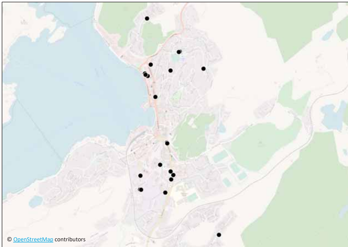
Figure 4.1 Location of properties in Oban where sewer flood depths are predicted (by Scottish Water modelling) to exceed 100 mm for a 1 in 200 year event (1 hour event duration).
