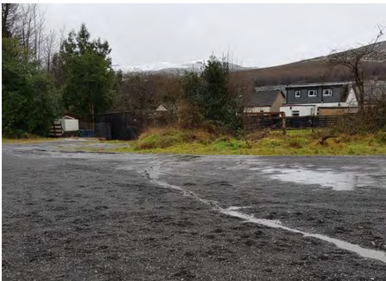
Figure 2-7: Overland flow path to south west corner visible during site walkover
