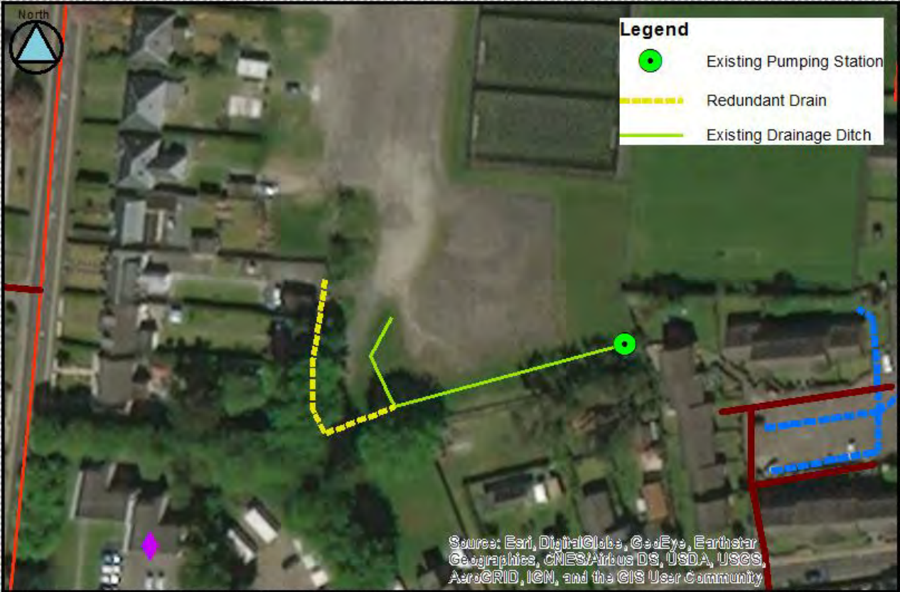
Figure 2-6: Existing drainage layout
