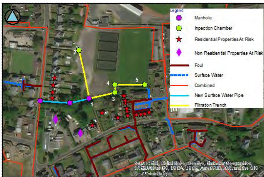
Figure 4-4: Outfall to combined sewer
