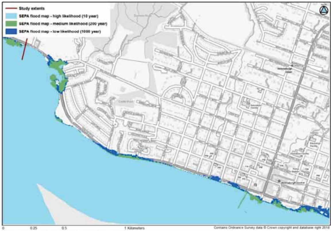
Figure 3-2: SEPA coastal flood extents (Helensburgh west)
