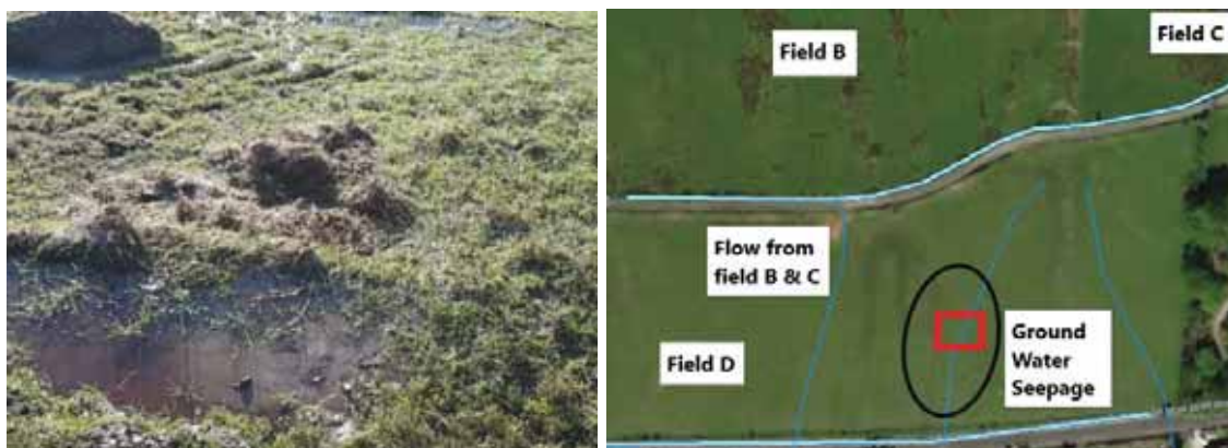
Figure 2-10: Typical ponding of ground water seepage possibly due to damaged pipe
