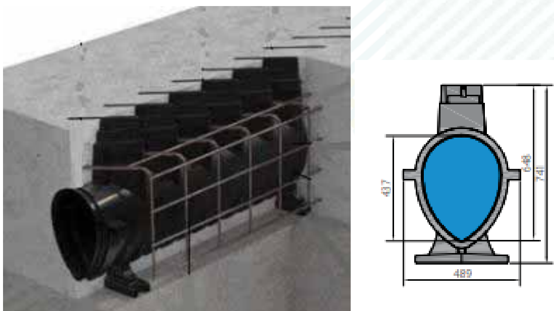
Figure 6-1: Drexus XL 425 installation and cross section
