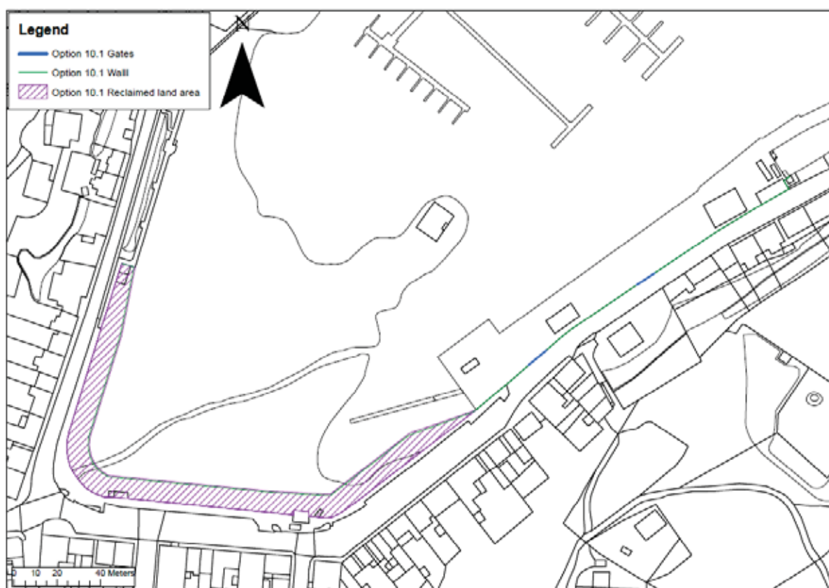
Figure 5-7 Option 10.1: Land reclamation and direct defence. Defence wall runs along the coastal side of reclaimed land, and landward side of harbour
