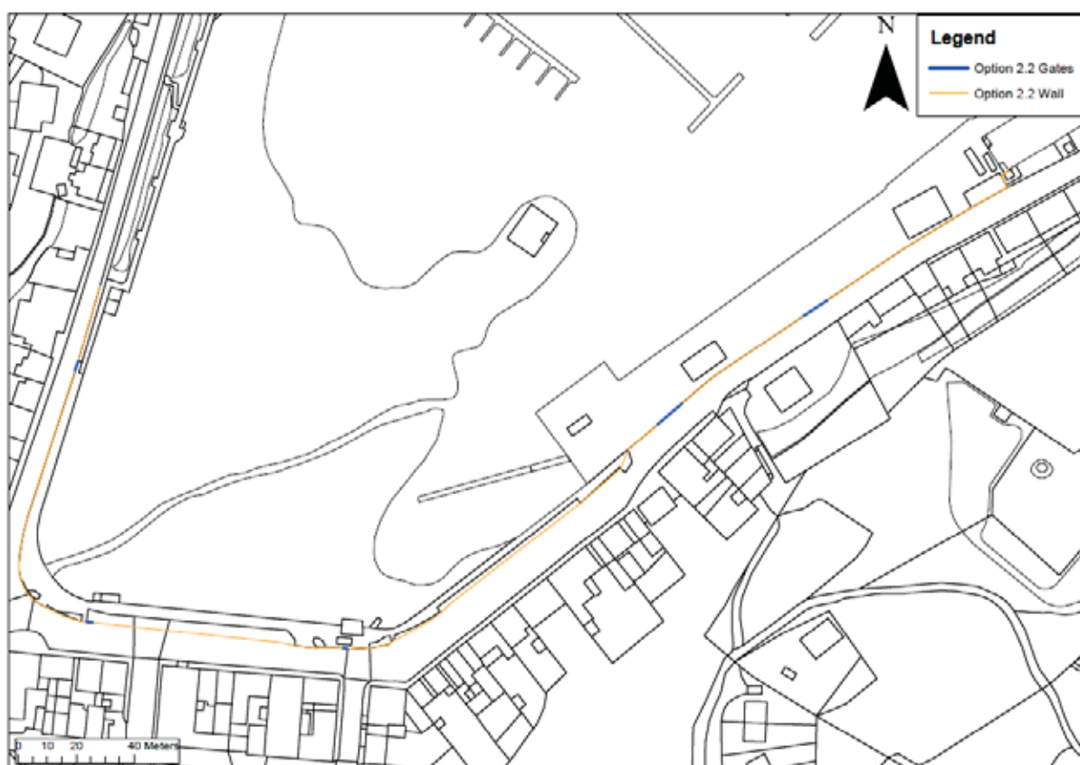
Figure 5-2 Option 2.2: Direct defence set back from existing harbour wall
